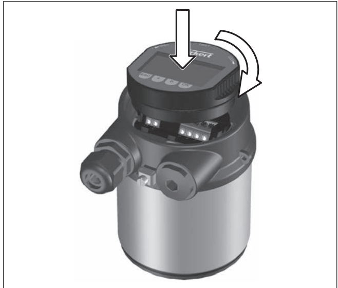
Fig. 30: Insertion of the display and adjustment module with single chamber housing
