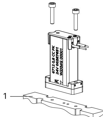
Fig. 1: Mounting the solenoid valve
