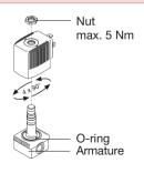
The coil can be rotated 4 x 90° (only 2 x 180° with block installation).
