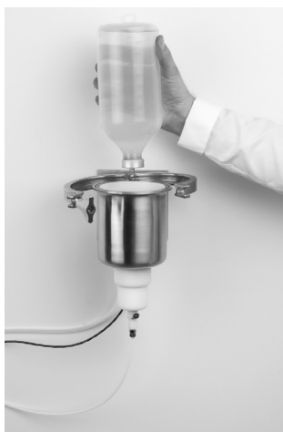
Fig 7: Insert electrolyte bottle
