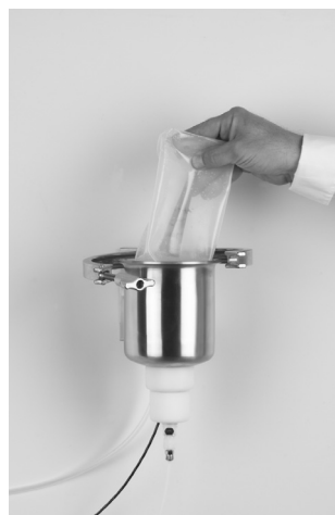
Fig 8: Remove electrolyte bottle
