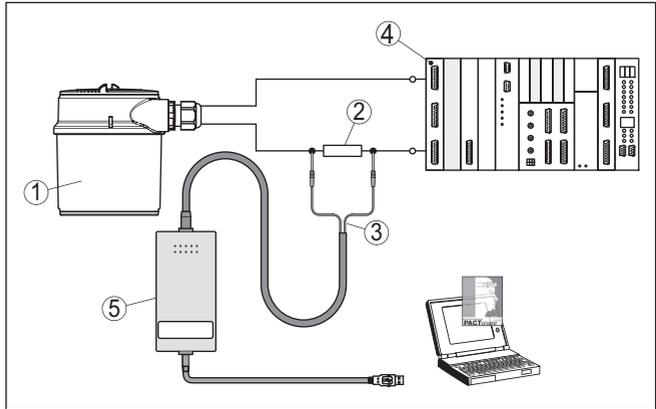
Fig. 12: Connecting the PC via HART to the signal cable
