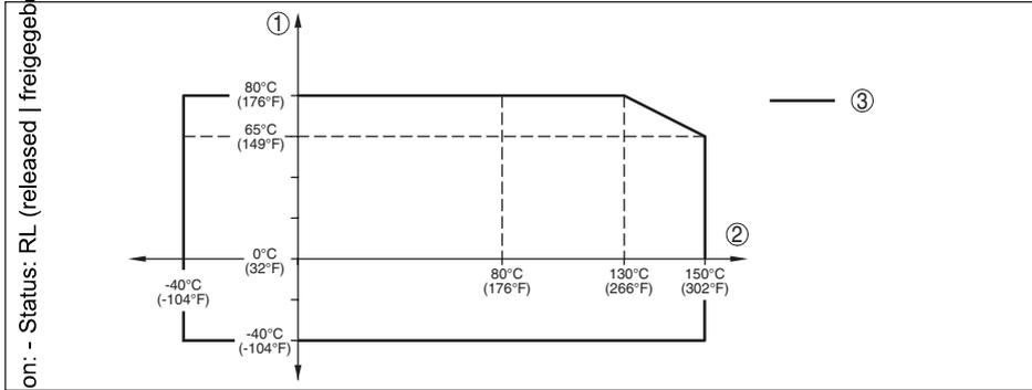
Fig. 28: Ambient temperature - process temperature, standard version
