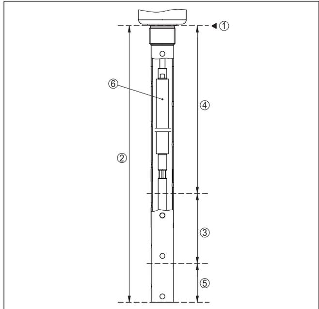
Fig. 6: Measuring ranges - LEVEL TRANSMITTER 8188 with steam compensation
