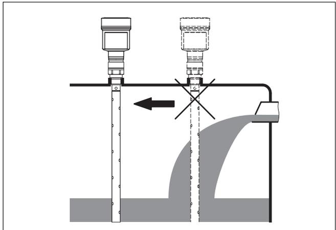
Fig. 5: Mounting of the sensor with inflowing medium
