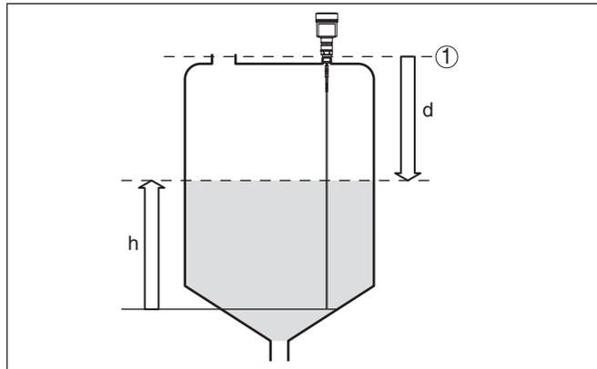
Fig. 2: Level measurement
