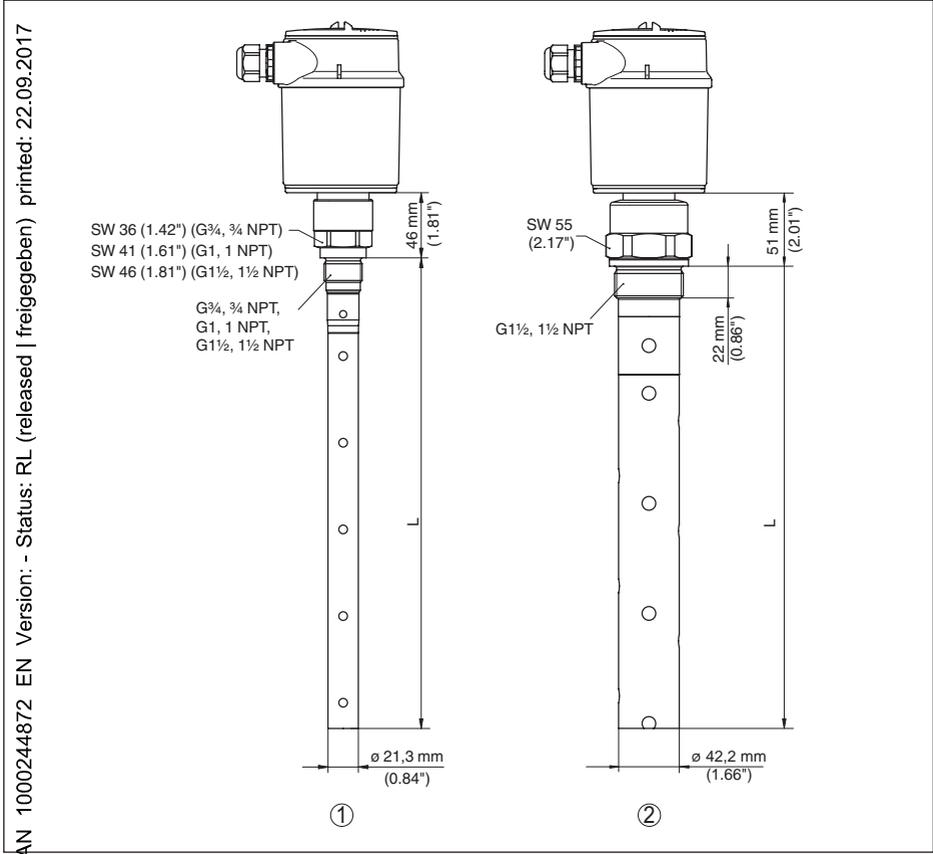
Fig. 32: LEVEL TRANSMITTER 8188, threaded version
