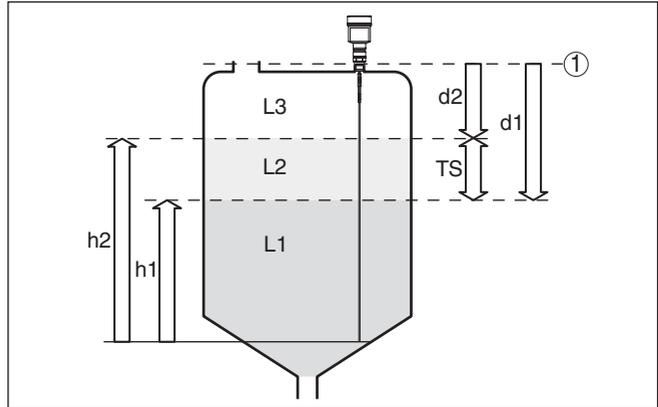
Fig. 3: Interface measurement
