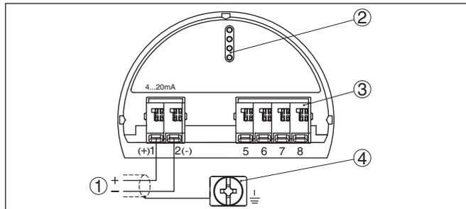
Fig. 8: Electronics and terminal compartment, single chamber housing
