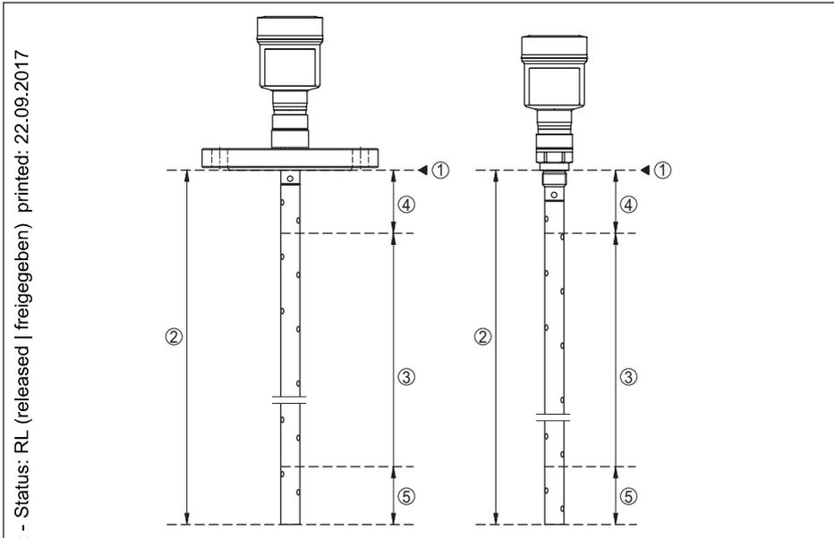
Figure 25: Measuring ranges - LEVEL TRANSMITTER 8188
