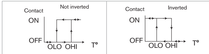
Fig. 26: Changing the output in hysteresis mode
